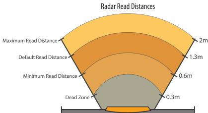
Radar detection range. Spanning from a 60° FOV from the e-loop, these are the range zones. The gray area is depicts the dead zone, in which objects cannot be detected. The Minimum read distance is 0.6m. The default read distance is 1.3m, and the Maximum read distance spans up to 2m.
