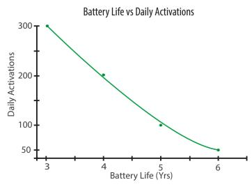
Note: Battery life is dependent on many factors, including daily activations, time used per activation, radar range and external conditions.
